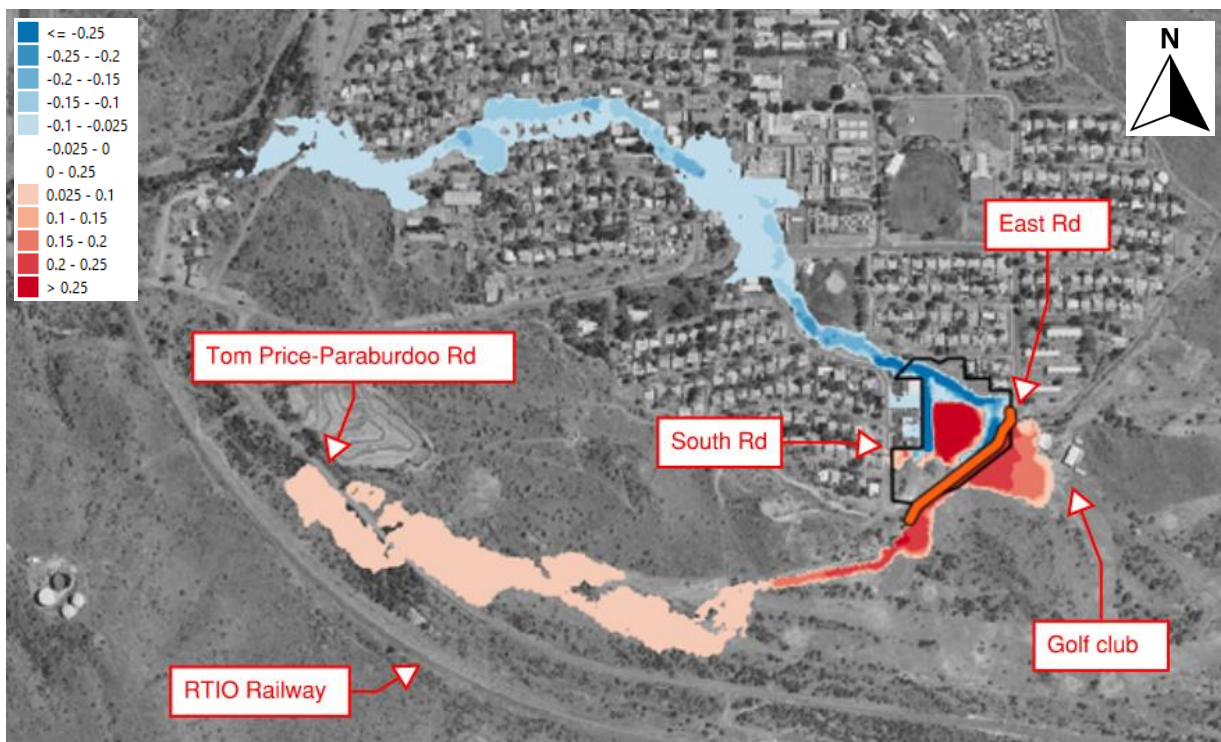
Figure 3-13: 1 in 100 AEP flood level differences (m) (2030 time horizon)
