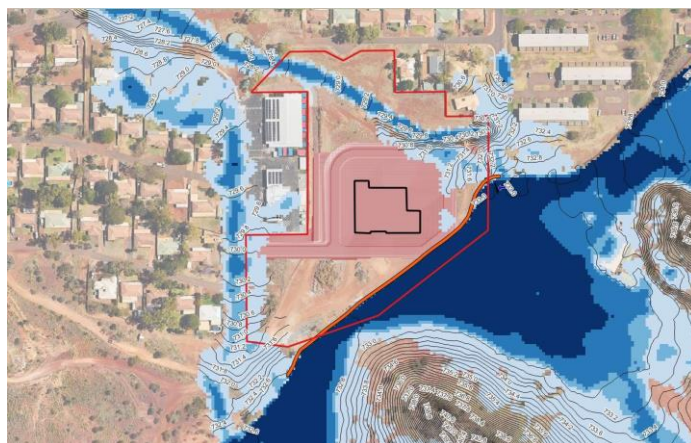
Figure 3-6: Design Option 3 – Full levee 1 in 500 AEP flood extent (1961-1990 climate scenario)
