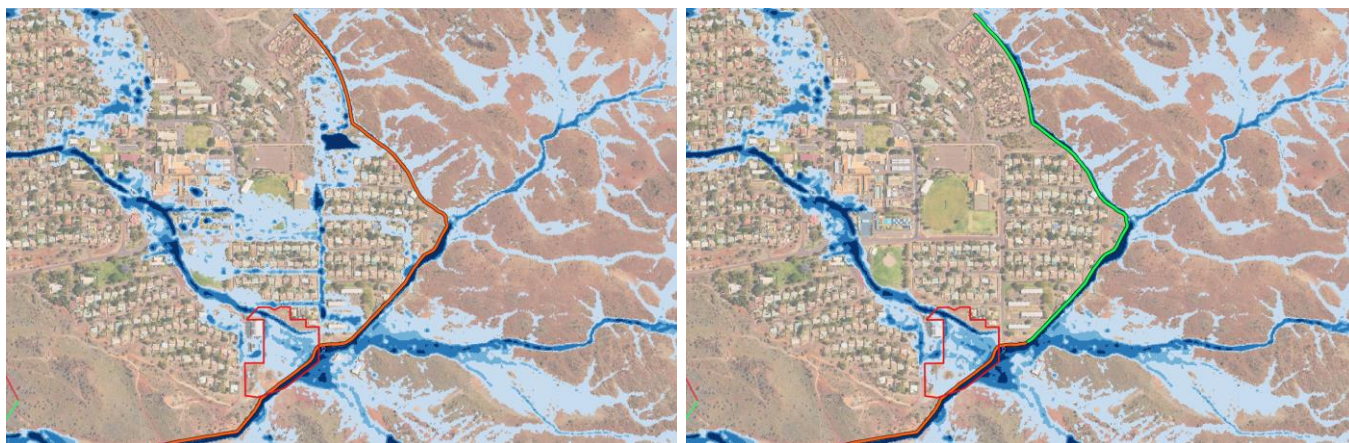
Figure 3-1: Existing informal bund along diversion drain (shown in orange) versus artificial levee scenario (shown in green)
