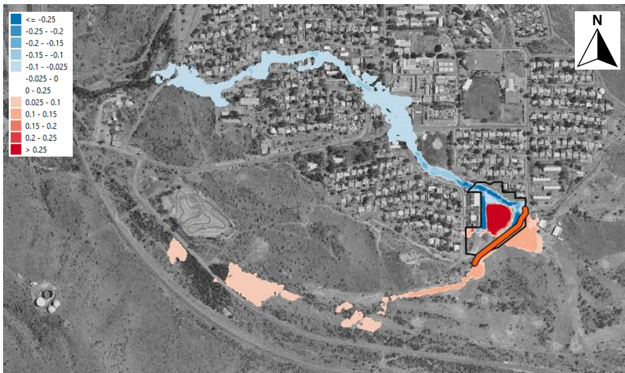
Figure 3-12: 1 in 20 AEP flood level differences (m) (2030 time horizon)
