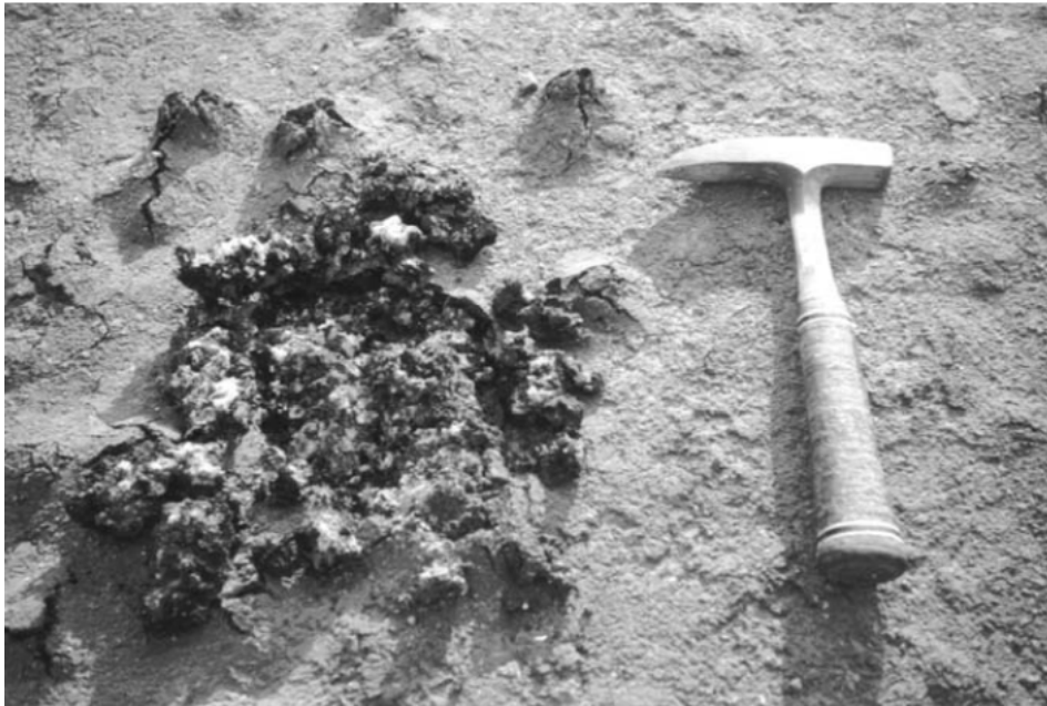
Figure 2.7: Volcano blisters and salt in loosened primed base
