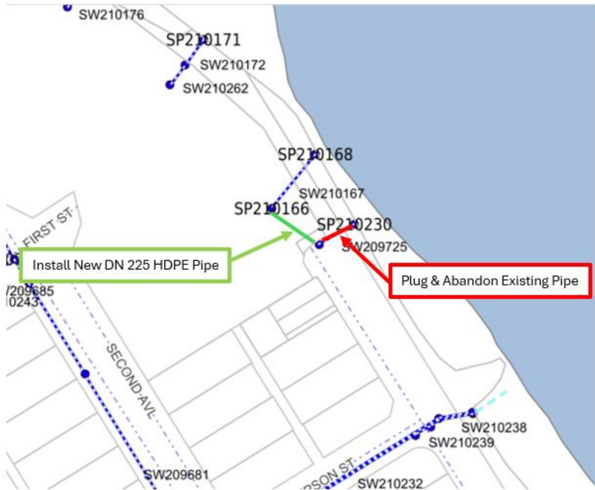
Figure 3. Decommissioning and Redirection of existing ocean outfall
