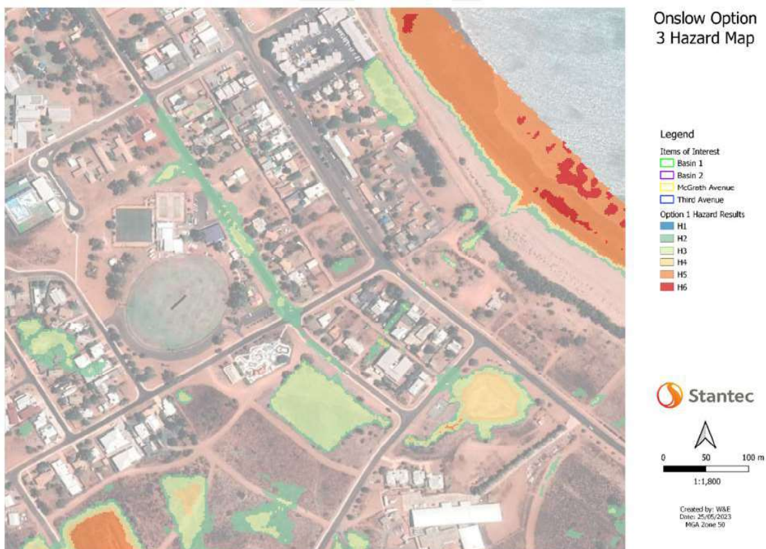
Figure 20 – 18-hour event Basin 1 Pump Hazard Classification
