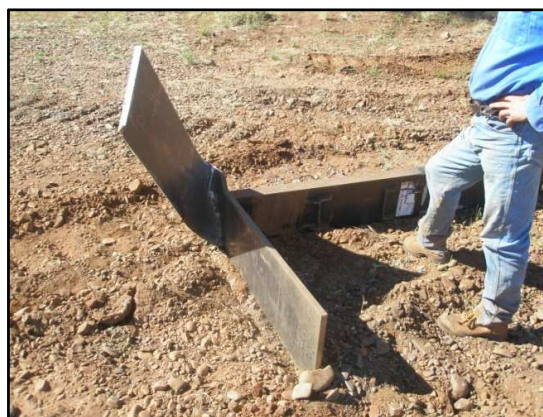
Above: Rear mounted, single wing blade plough behind a D9 Dozer, damage to wing resultant from a stubborn root
