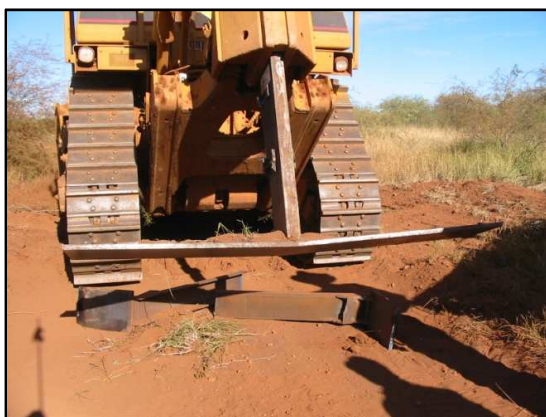
Above: Rear mounted, single wing blade plough behind a D9 Dozer, damage to wing resultant from a stubborn root
