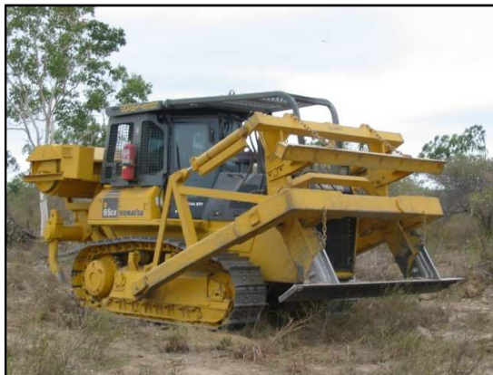
Above: Dozer @ Urala Station with front mounted cutter bar (stick rake), Ellrott Plough® in Queensland
