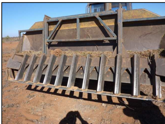
Above: Dozer @ Urala Station with front mounted cutter bar (stick rake), Ellrott Plough® in Queensland
