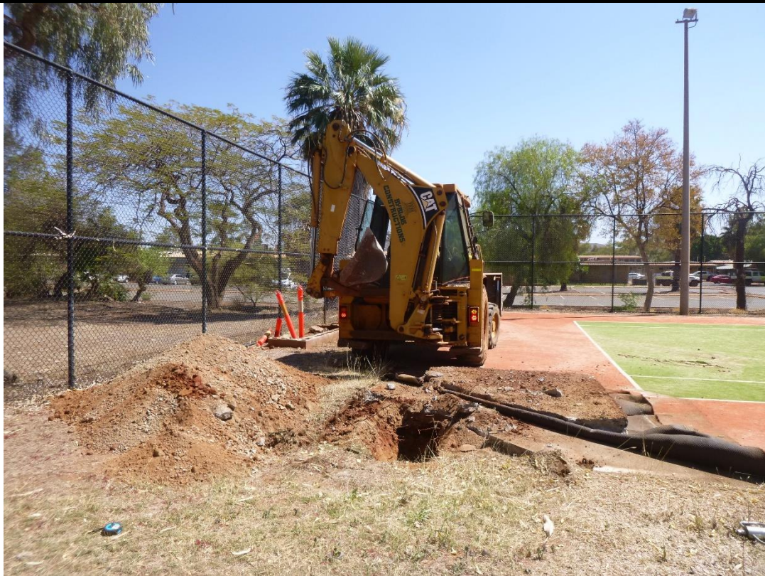
Photo 5. Test Location 02 (TP2), Sub-surface probing by using an excavator
