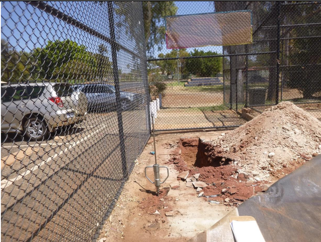
Photo 10. Test Location 04 (DCP4), Testing by a Dynamic Cone Penetrometer
