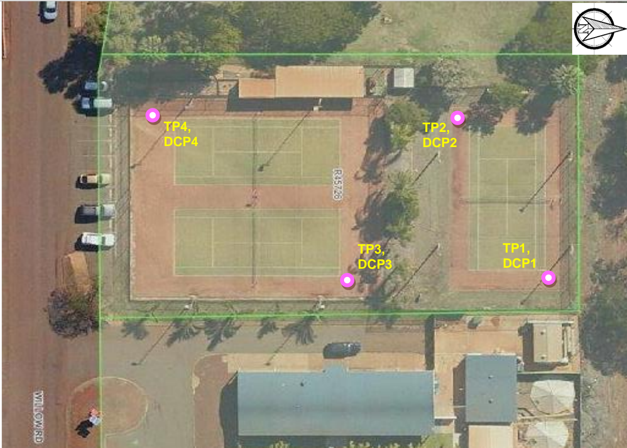
Site Sketch : Test Pit and Dynamic Cone Penetrometer Test Locations
