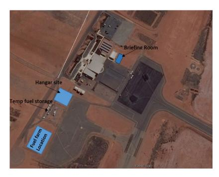
The hangar is designed to house 2 x S-92 helicopters and will have both airside access to the General Aviation apron plus landside access to the road at the rear of the allotments.
